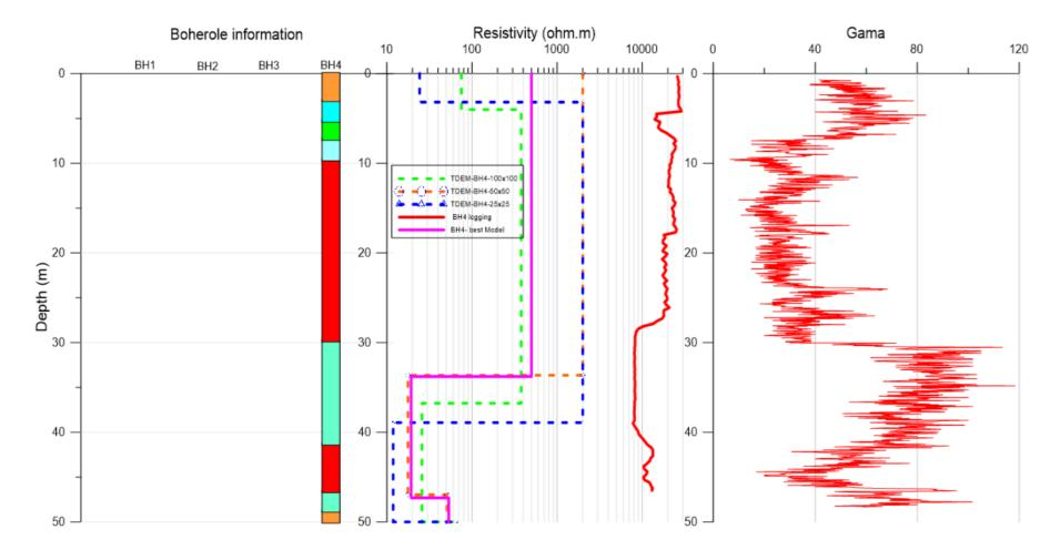
TDEM sounding interpretation allows us to locate thick clayey layer between 33 and 47 m deep, also detected
