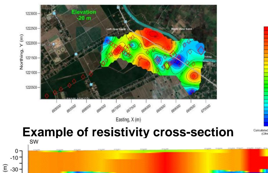
TDEM resistivity map at 20 m deep allows us to delineate the clayey layer (in blue) and sandy aquifer (in red). Clayey layers are not connected between eachothers,
